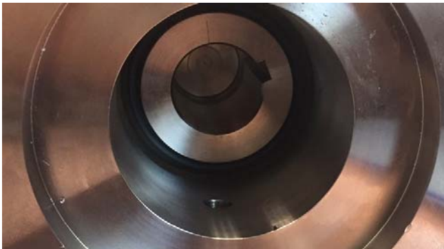
Figure 3 - View of Gearbox-to-Pump interface, including adapter piece (view looking at gearbox)
